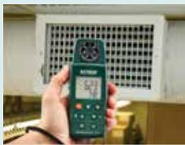
Measure Air Velocity, Air Flow, Air and Type K Temperature, Heat Index, Humidity, Wet Bulb, Dew Point, Windchill, and Light Level. Includes low friction ball bearing mini vane wheel, a precision photo diode with cosine and color correction
