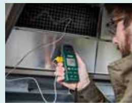
Convenient 4-in-1 Anemometer measures Air Velocity, Air Flow, Air Temperature, and Type K Temperature. Built-in low friction ball bearing mini vane wheel for high accuracy. General purpose
