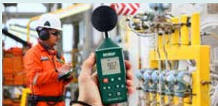
Compact design with  $\pm 1$ dB high accuracy and a large backlit display provides quick and reliable sound level testing. It meets Class 2 standards (IEC 61672-2013 and ANSI/ASA S1.4/Part 1). Measure A & C weighting from 35 to 130dB with Fast and Slow response time selectivity.
