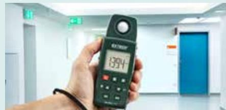
Measures light intensity up to 1860 Foot-candles (20,000 Lux) with resolution to 0.1 Fc/1Lux. Ideal for indoor lighting tests and for checking security and safety illumination in parking garages, night time ATM areas, stairwells, landings, and hallways.
